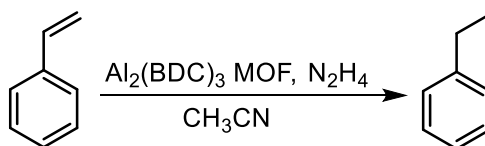
Scheme 1.1. \text{Al}_2(\text{BDC})_3 MOF catalysed hydrogenation of olefins.
