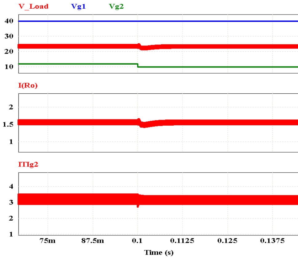
Fig. 4. 92 The variation of V_o and I_{g2} currents when V_{g2} : 12V to 10V
